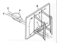
Install ring (4) on backboard(6) by 4pcs bolt(2), also install backboard bracket(7) on backboard (6) by bolt(1) as shown.
