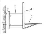
Fix the 2pcs backboard bracket (7) by plug bolt (3) on wall as shown.
