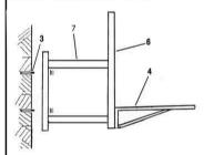
1. Fix the 2pcs backboard bracket (7) by plug bolt (3) on wall as shown.
