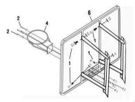
2.Install ring (4) on backboard(6) by 4pcs bolt(2), also install backboard bracket(7) on backboard (6) by bolt(1) as shown.
