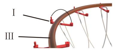
2 II. Snap into the groove of the hoop (III.), as shown in the figure
