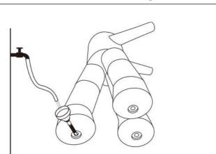
3. Fill water into the three designated positions using a funnel. screw the cap back on with the hex wrench.
