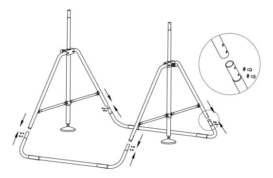
The horizontal bar grip connected with the adjustable bar, and then lock the screw
