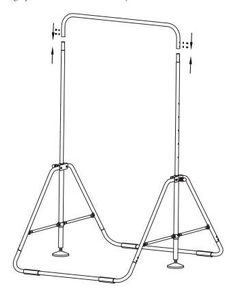
Five speed adjustments, adjust the height from 90cm to 130cm
