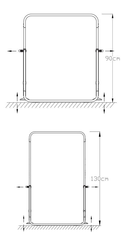
When there is a gap between base flate and the ground, spin the adjustment to reach the ground
